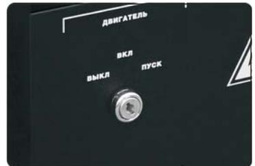
(c) Set the engine switch to "OFF" position.
