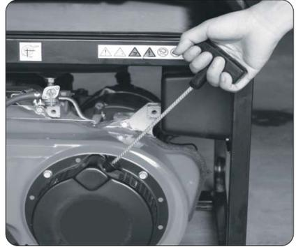
(e) After the engine started, return the choke lever gradually to "OPEN" position.
